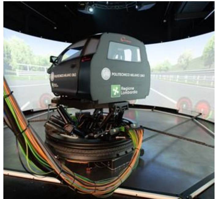
FIGURE 2: DRIVING SIMULATOR AT DRISMI LABORATORY OF POLTECNICO DI MILANO
